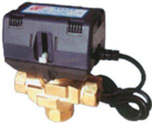
ABC20 series of Motorized Valve is used to control the on-off conversion of Heating Air Condition Water System, it is consist of a driver and a valve body .The driver adopts the synchronous motor to make its performance more stable and prevent the water hammer.
