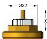
TA-COMPACT-T is developed to work together with the EMO T actuator. Actuators of other brands require a working range of X (closed - fully open) = 11,6 - 15,6 and an adjusting force of 125 N.
